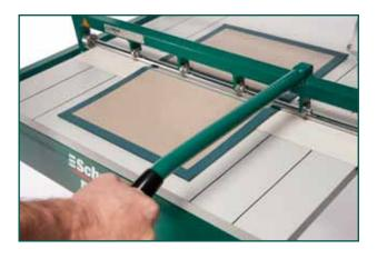
Rounding on a flexible base is something very special as it prevents the spine from cracking and allows very even rounding of the whole spine hollow. Moreover, the pressure put on the spine during the rounding process prevents the spine hollow from coming off the cover material.
