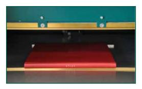
stop which is adjusted to the book size. The stop is released by push-button, aligned according to the book width and fixed at the correct position by the push-button. All further books is pushed against the stop only and is aligned properly.
