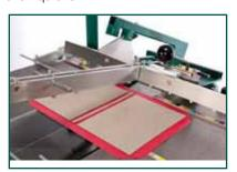
After the cover has been aligned, the guide angle with the spine hollow is lowered by means of air pressure. While the spine hollow is pressed down by the blade, both boards are placed manually into the guide angles and pressed down for a moment. The guide angles can then be lifted, and the case is ready to be turned in, for example on our **PräKant** turning-in machine.
