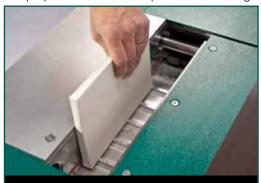
its spine facing downwards and is secured with a pressing plate. The latter is moved by a foot pedal.
