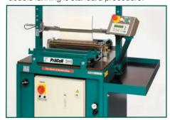
When the gluing process is finished, the clamp is unlocked. The second operator lifts the clamp and turns it so that the freshly glued spine of the book block faces upwards. The front edge of the book block is now pressed in the clamping station underneath the drying clamp. The drying clamp is opened lightly, lifted up pressed together by hand right underneath the glued spine. Now, a mull may be applied manually.
