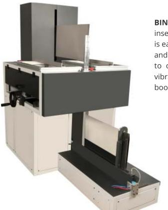
**BINDWEL CASING-IN** machine ideally for the perfect inserting of book block in the finished case. Machine is easy to operate and maintain. With the pneumatic and PLC technology to travel the book from one place to other. Easy make ready and operating. Non vibrating heavy machine for accurate place of the book in to the cases.
